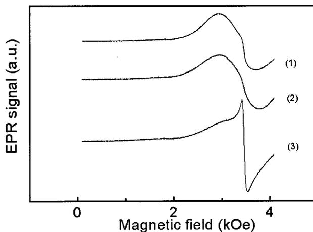
FIG. 1. Room temperature EPR spectra of nanoparticles: Fe<sub>2</sub>O<sub>3</sub> (curve 1), BaFe<sub>2</sub>O<sub>4</sub> (curve 2), and BaFe<sub>12</sub>O<sub>19</sub> (curve 3).
