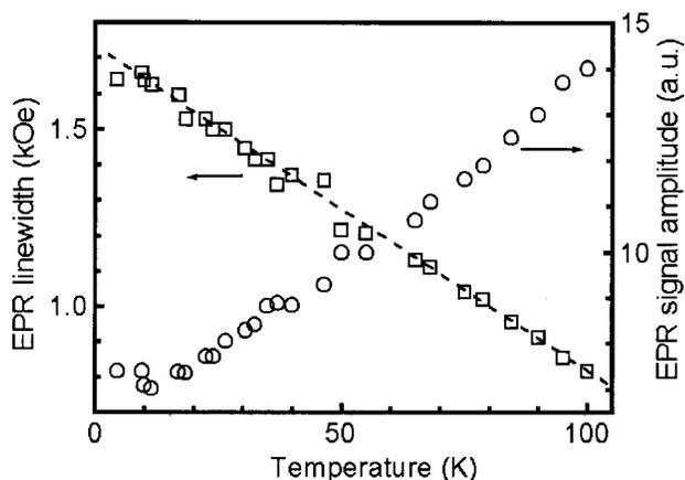
FIG. 7. Thermal variation of the EPR amplitude (circles) and linewidth (squares, dashed line) for the  $\text{BaFe}_{12}\text{O}_{19}$  nanoparticles. The line is a guide for the eye.
