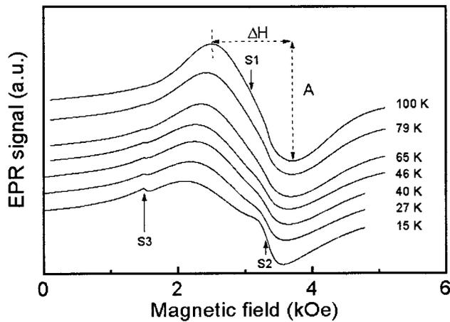
FIG. 2. EPR spectra of  $\text{Fe}_2\text{O}_3$  nanoparticles at different temperature.  $\Delta H$  is the peak-to-peak linewidth,  $A$  is the EPR signal amplitude. It is presumed that S1 is the superparamagnetic signal ( $g=2.12$ ) from the  $\gamma\text{-Fe}_2\text{O}_3$  phase, S2 is the paramagnetic EPR signal ( $g=2.02$ ) from magnetically isolated centers in  $\gamma\text{-Fe}_2\text{O}_3$ , S3 is the rhombic symmetry signal ( $g=4.3$ ) from the  $\alpha\text{-Fe}_2\text{O}_3$  phase.
