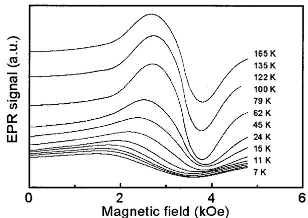
FIG. 5. EPR spectra of the  $\text{BaFe}_2\text{O}_4$  nanoparticles at different temperatures.
