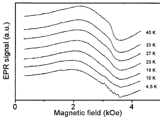
FIG. 8. Low-temperature EPR spectra of  $\text{BaFe}_{12}\text{O}_{19}$  nanoparticles.
