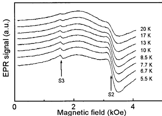
FIG. 3. EPR spectra of  $\text{Fe}_2\text{O}_3$  nanoparticles at low temperatures.
