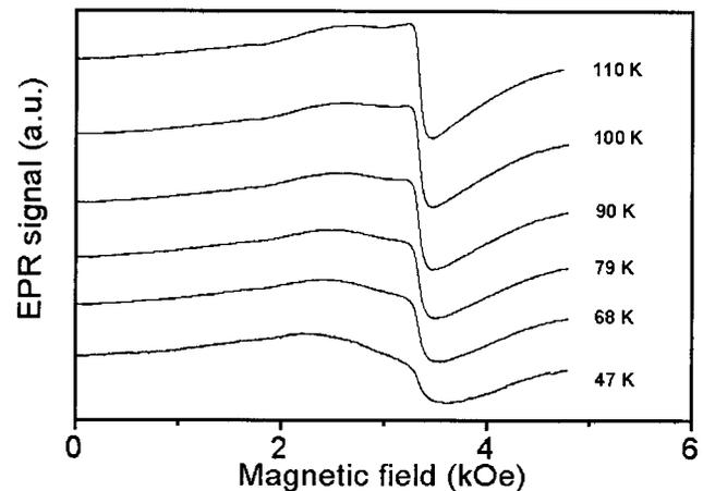
FIG. 9. EPR spectra of  $\text{BaFe}_{12}\text{O}_{19}$  nanoparticles at different temperatures.
