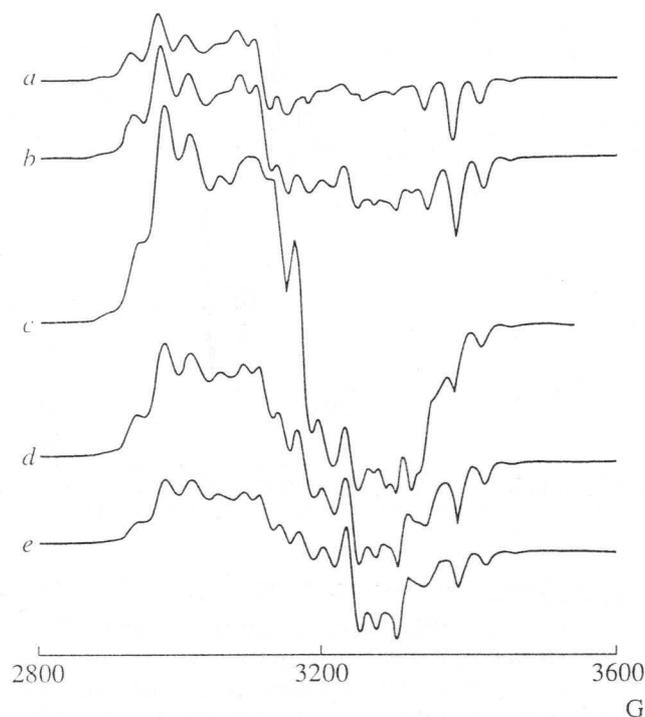
Fig. 2. EPR spectra (77 K) of the products of oxidation of the Pt(IV) hydroxo complex in NaOH ( $c_{\text{OH}^-} = 5 \text{ mol/l}$ ) by excess  $\text{Na}_2\text{S}_2\text{O}_8$  at  $100^\circ\text{C}$  for (a) 1, (b) 3, (c) 10, (d) 20, and (e) 40 min.
